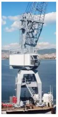
Cranes of YHV series are suitable for floating dock applications. Handling of hook loads for general ship repair and maintenance works are common operation modes. Typical of the YHV type crane design is the narrow rail span length and the feature to luff the jib down to rail level during towing of the dock on open seas. Floating dock cranes are the main power of ship repair yards and therefore shall be carefully engineered to achieve its duties.
