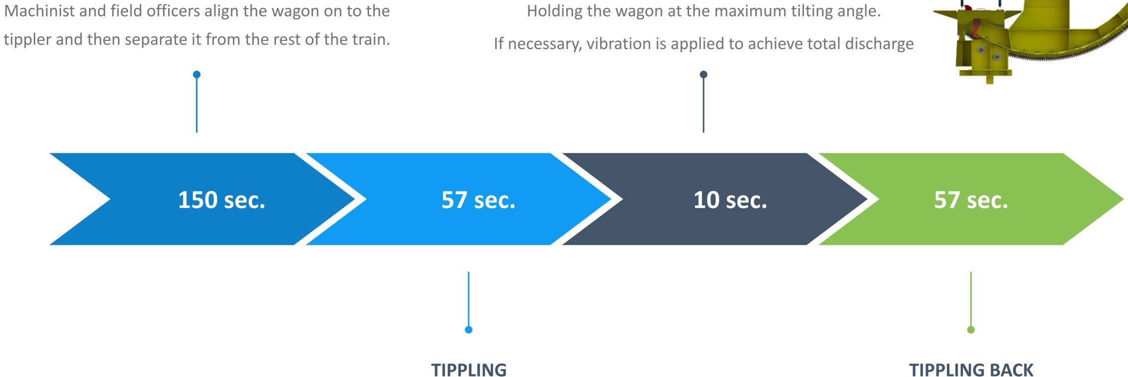
The wagon to be emptied gets clamped with hydraulic arms and simultaneously gets turned by 160 degrees.
